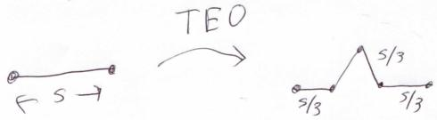
The Koch snowflake is constructed by beginning with an equilateral triangle then applying the TEO infinitely often.
